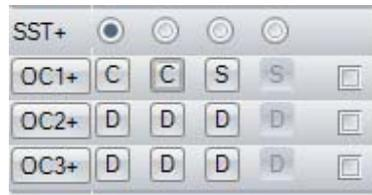
Both Settings would require “AR On” to be enabled, otherwise they both would act as a single shot operation. Reclosers would trip straight to lockout, and Sectionalisers would operate on the first fault passage and isolation.
