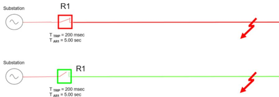
*Traditional Recloser Sequence (top down) under limited grading scenario – Fault causes isolation of entire feeder below protecting recloser.*
